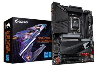
Z790 AORUS ELITE AX DDR4 Scheda madre - Supporta processori Intel Core 14th Gen CPUs, 16+1+2 Phases Digital VRM, up to 5333MHz DDR4 (OC), 4xPCIe 4.0 M.2, Wi-Fi 6E, 2.5GbE LAN, USB 3.2 Gen 2x2
