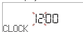
Turn the *adjustment knob* to set the current hour and press  $\checkmark$ : The two digits for the minutes will flash on the display. Turn the *adjustment knob* to set the minutes and press  $\checkmark$  to confirm.
