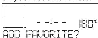
If you would like to save a function as a favorite and store the current settings for future use, press  $\checkmark$  otherwise, to ignore the request press  $\ll$ . Once  $\checkmark$  has been pressed, turn the *adjustment knob* to select the number position, then press  $\checkmark$  to confirm.
