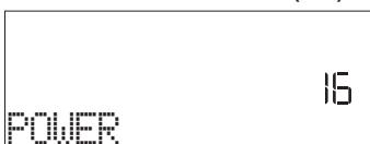
Turn the *adjustment knob* to select 16 "High" or 13 "Low" and press  $\checkmark$  to confirm.
