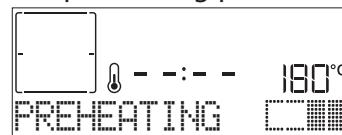
Once this phase has finished, an audible signal will sound and the display will indicate that the oven has reached the set temperature, requiring to "ADD FOOD".
