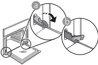
2. Close the door as much as you can. Take a firm hold of the door with both hands – do not hold it by the handle. Simply remove the door by continuing to close it while pulling it upwards at the same time until it is released from its seating. Put the door to one side, resting it on a soft surface.
