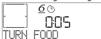
An audible signal will sound and the display shows the action to be done. Open the door, do the action prompted by the display and close the door, then press
