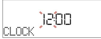
Press + or – to set the current hour and press ✓: The two digits for the minutes will flash on the display. Press + or – to set the minutes and press ✓ to confirm.
