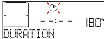
When the ⌚ icon flashes on the display, press + or – to set the cooking time you require and then press ✓ to confirm. You do not have to set the cooking time if you want to manage cooking manually (untimed): Press ✓ or ⏻ to confirm and start the function. By selecting this mode, you cannot program a delayed start.
