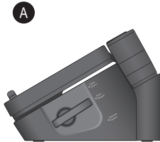
Push Latch into Store position to store.
