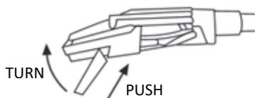
To reposition the stylus, hold the sides of the red stylus holder, make sure the stylus is facing downwards, and gently push the holder at a minimal angle towards the head at the end of the tonearm until it is securely fastened.
