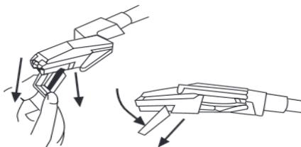
To remove the stylus, firmly grasp the tonearm and plastic stylus holder with two fingers and gently pull the red stylus holder towards you, away from the cartridge.
