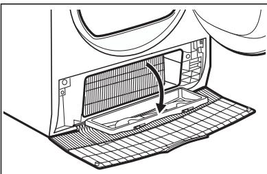
5. If necessary, remove the fluff from the condenser and its compartment. You can use a vacuum cleaner with a brush attachment.
