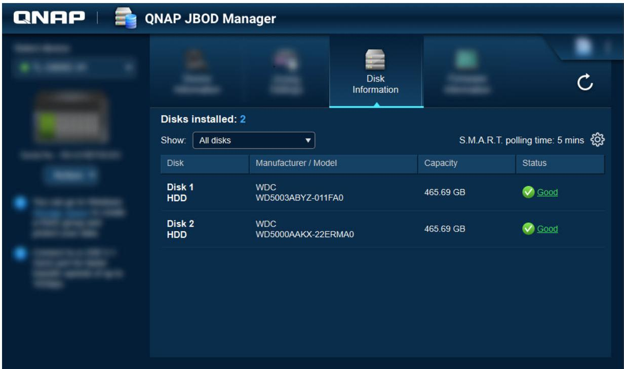
The screenshot shows the QNAP JBOD Manager interface. The 'Disk Information' tab is active, displaying 'Disks installed: 2'. A dropdown menu is set to 'All disks' and the S.M.A.R.T. polling time is 5 mins. The table below shows the following data:
