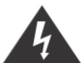
The lightning flash with arrowhead symbol, within an equilateral triangle is intended to alert the user to the presence of insulated 'dangerous voltage' within the product's enclosure that may be of sufficient magnitude to constitute a risk of electric shock to persons.
