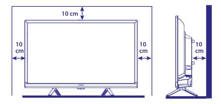
Install the display on a solid horizontal surface such as a table or desk. For ventilation, leave a space of at least 10 cm free all around the set. To prevent any fault and unsafe situations, please do not place any objects on top of the set. This apparatus can be used in tropical and/or moderate climates.
