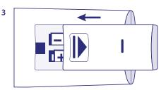
Place 2x AAA batteries in the battery compartment of the remote control. Make sure to match the polarity markings inside the compartment.
