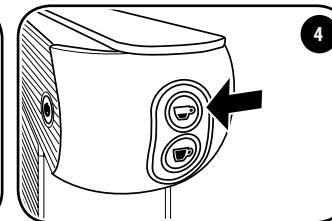
Make sure that there are no E.S.E.pods inside the machine, and switch it ON using the main switch.
