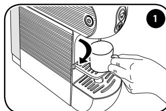
Lower the support to prepare an espresso coffee correctly, and to use espresso cups.
