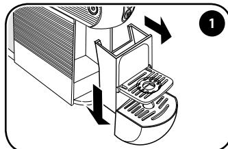
To perform this operation, remove the tray and separate it from the E.S.E. pod drawer by pushing it downwards; be aware that there may be liquid in the tray.
