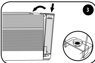
Insert the tank by tilting it slightly and placing it on the water valve. Press the upper part into the machine until a click is heard.
