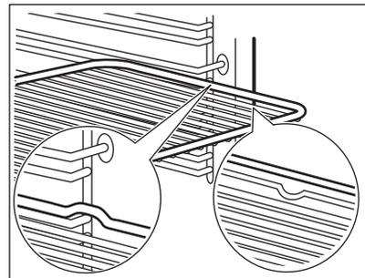
Insert the shelf between the guide bars of the shelf support and make sure that the feet
