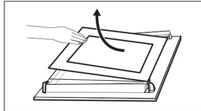
8. Clean the glass panels with water and soap. Dry the glass panels carefully. Do not clean the glass panels in the dishwasher.
