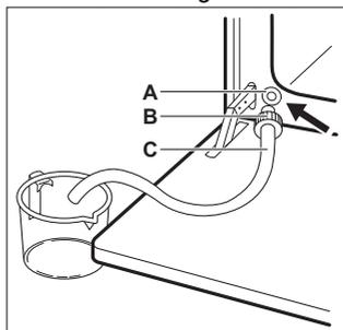
3. Keep the end of the pipe below the level of **A** and push **B** repeatedly to collect remaining water.
