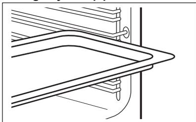
Push the tray between the guide bars of the shelf support. Place the baking tray with the slope towards the back of the oven interior.
