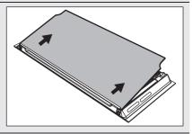
Step 5 Pull the front part upwards. The 4 pins detach from their housings.
