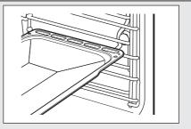
i) The mechanical safety locks that prevent the wire shelf from being removed accidentally should face downwards and towards the back of the oven cavity.
