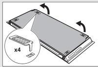
**Step 6** Remove the intermediate glass by lifting it upwards.
