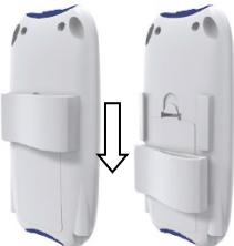
2) Remove battery cover by pulling on tag.
