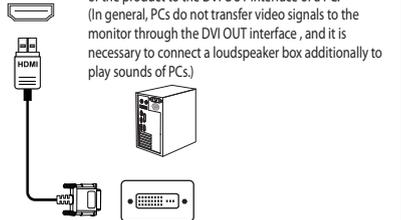
Use the HDMI-DVI cable to connect the HDMI IN interface of the product to the DVI OUT interface of a PC. (In general, PCs do not transfer video signals to the monitor through the DVI OUT interface, and it is necessary to connect a loudspeaker box additionally to play sounds of PCs.)
