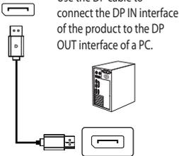
Use the DP cable to connect the DP IN interface of the product to the DP OUT interface of a PC.
