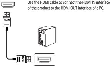
Use the HDMI cable to connect the HDMI IN interface of the product to the HDMI OUT interface of a PC.
