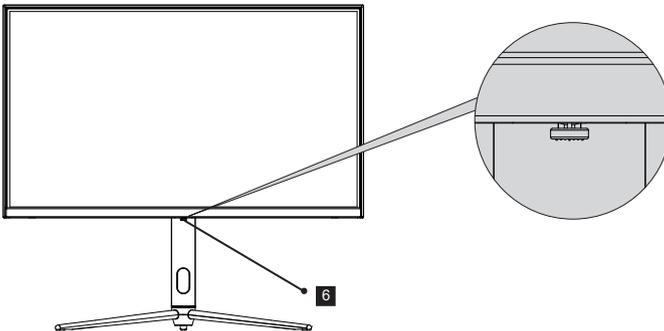
6. Indicator: Steady blue light indicates that power is on and the monitor is operating normally. A red light indicates no video source, no horizontal or vertical signal detected or low voltage. No light indicates a shutdown condition. Make sure your computer is turned on and that all video cables are fully plugged in and/or connected.
