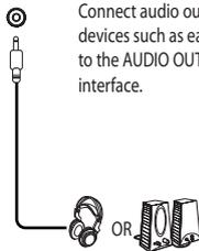
Connect audio outputting devices such as earphones to the AUDIO OUT interface.
