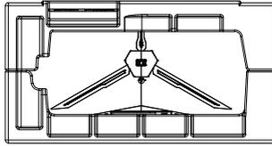
2. Use 2 screws to lock the shaft assembly and bracket, and then lock 3 screws to the base.
