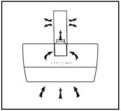
Activated carbon filter can be used to trap odors.
