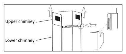
◆ Drill 2×8mm holes to accommodate the plate II. Screw and tighten the plate II onto the wall with 2 screws provided. Assembly the chimney onto the unit and fix it with 2 screws.
