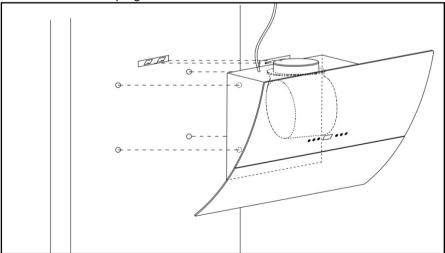
• Fix the one-way-valve to the air outlet of the cooker hood. Then, attached the exhaust pipe onto the one-way-valve as shown below.
