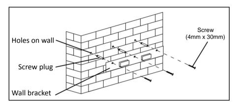
• For inclined panel Model, need to drill 4 x 8mm extra holes & fixing screws & screw plugs before installation.
