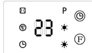
The timer is also a start programmer when the appliance is in stand-by: every time the button gets pressed the timer adds one hour of stand-by, when the time runs out the appliance starts automatically. The remaining time (in hours) is written on the display until the time runs out and
