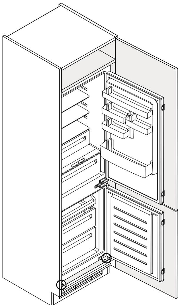
Using the screws provided, attach the feet to the bottom shelf.
