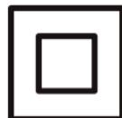
This appliance has been designed with a double-insulation system for your safety. **CE**
