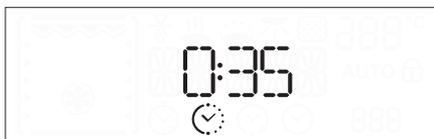
Press  $\frac{OK}{select}$  to set the end time of the cleaning cycle or to activate the function.
