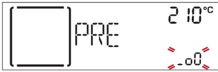
Once this phase has finished, an audible signal will sound and the display will indicate that the oven has reached the set temperature:
