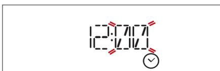
Turn the *adjustment knob* to set the minutes and press **OK select** to confirm.
