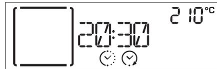
Notes: Programming a delayed cooking start time will disable the oven preheating phase: The oven will reach the temperature you require gradually, meaning that cooking times will be slightly longer than those listed in the cooking table.
