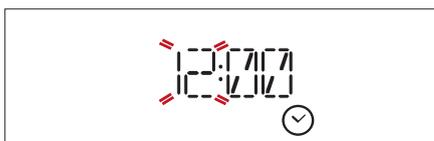
Turn the *adjustment knob* to set the correct hour and press **OK select**: The two digits for the minutes will flash on the display.
