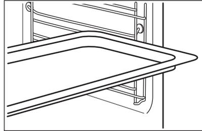
Push the tray between the guide bars of the shelf support. Place the baking tray with the slope towards the back of the oven interior.
