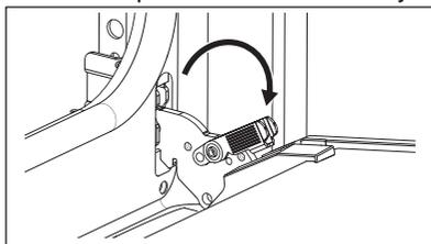
3. Close the oven door halfway to the first opening position. Then lift and pull to remove the door from its seat.
