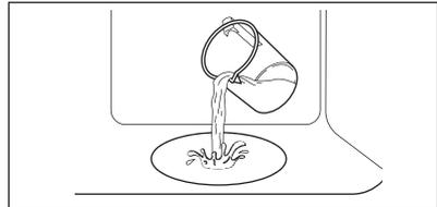
The maximum capacity of the cavity embossment is 250 ml. Do not refill the cavity embossment during cooking or when the appliance is hot.
