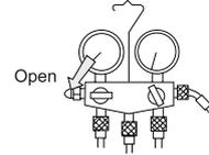
3. Vacuumize for over 15min. And check the level gauge which should read - 0.1MPa (-76 cm Hg) at low pressure side. After the completion of vacuumizing, close the handle 'Lo' in the vacuum pump. Check the condition of the scale and hold it for 1-2min. If the scale-moves back in spite of tightening, make flaring work again, then return to the beginning of the step 3.
