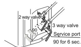
5. No gas leakage? In case of gas leakage, tighten parts of pipe connection. If leakage stops, then proceed the step 6. If it does not stop gas leakage, discharge whole refrigerants from the service port. After flaring work again and vacuumize, fill up prescribed refrigerant from the gas cylinder.
