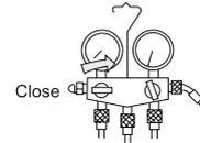
4. Open the valve rod for the 2-way valve to an angle of anticlockwise 90 degree. After 6 seconds, close the 2-way valve and make the inspection of gas leakge.
