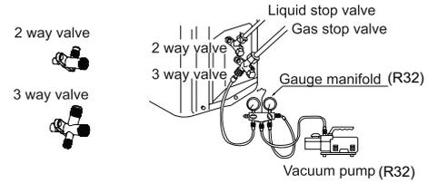
2. Open the handle at low in gaugemanifold, and operate vacuum pump. If the scale-moves of gause (low) reach vacuum condition in a moment, check the step 1 again.
