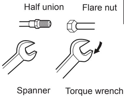
Forced fastening without careful centering may damage the threads and cause a leakage of gas.
