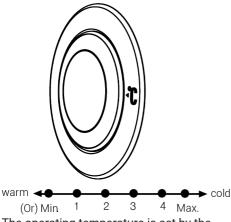
The operating temperature is set by the temperature control.
