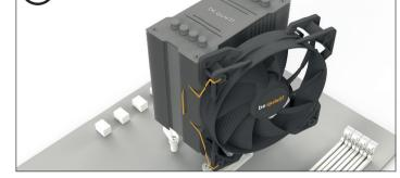
Fasten the 120mm fan (2) onto the cooler unit (1) using fan clips (15). Connect the fan to the motherboard's PWM signal.
