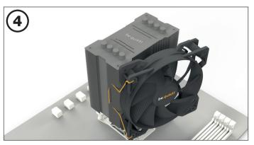
Fasten the 120mm fan (2) onto the cooler unit (1) using fan clips (15). Connect the fan to the motherboard's PWM signal.
