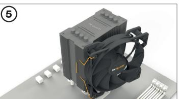
Fasten the 120mm fan (2) onto the cooler unit (1) using fan clips (15). Connect the fan to the motherboard's PWM signal.
