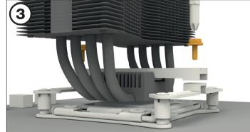
Position the cooler mounting bridge (6) centrally on the cooler (1). Next place the cooler unit onto the CPU. Insert the mounting bridge fastening screws (11) from above into the cooler mounting bridge and then screw these alternately tight. You can use any cross-tip screwdriver for this.
