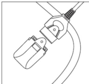
Make sure there is a power outlet nearby and that the power cord is not in a position that could constitute a tripping hazard. When connected to the mains, the power supply unit must be within easy reach of the user. Do not cover the power unit and do not apply pressure to it.
