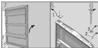
7. Lift the loose refrigerator door carefully off the lower hinge.
