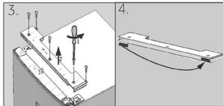
3. Remove the five screws which fix the front panel (1) and remove the panel (2).
