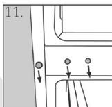
11. Change the positions of the blanking plugs and the screw on the side.
