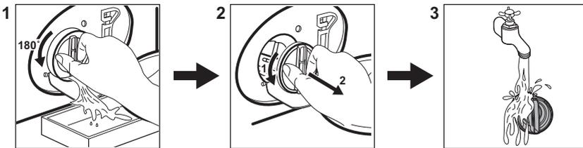
Clean the filter regularly and, especially, if the alarm code **E20** appears on the display.
