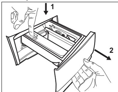
2. Remove the top part of the additive compartment to aid cleaning. Make sure that all detergent residue is removed from
