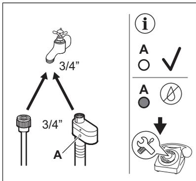
5. Connect the other end of the COLD water inlet hose to the cold water tap with 3/4" thread.
