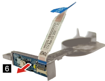
Figure 34. Disconnect and remove the power board with cable
