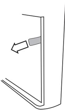
3. Pull out the pre-filter. Now, to pull out the combi filter, pull carefully on the side tabs.
