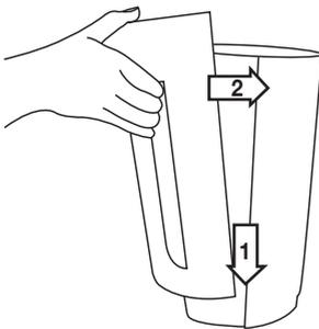
5. Re-insert the housing cover as shown until you see and hear it click into place (magnetic fastening). First attach the magnetic fastening at the bottom, and then at the top.
