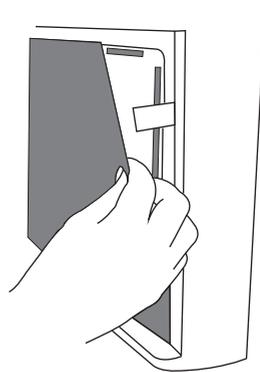
4. Insert a new combi filter. To insert the combi filter correctly, align it with the tabs as shown. Position the pre-filter above it.
