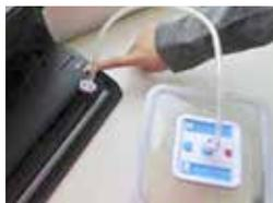
4. Take the provided vacuum hose and connect the narrow adapter plug to the vacuum port at the right side of the appliance. The adapter plug must be attached securely and should not be able to slip off. Place the other end of the vacuum hose onto the middle hole on the lid of the 4-angled container (art.no.: 46111).
