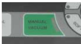
If you want to vacuum step by step and seal at a later time, press the »MANUAL Vacuum« button. You can determine yourself how much is to be vacuumed - eg for sensitive foods. Press and hold the button - the indicator light illuminates green - the appliance is vacuuming. Release the button, the appliance will
