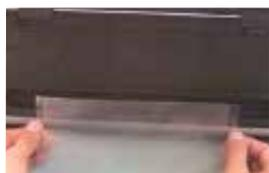
4. Place one open end of the foil on the sealing strip. The end of the foil does not need to extend over the black foam rubber seal into the vacuum chamber, because there is no need to operate the vacuum pump for sealing the bottom of the bag.
