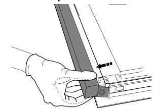
**2.** Lift and firmly hold the inner glass with both hands, remove it and place it on a soft surface before cleaning it.
