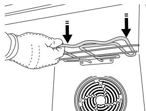
2. To return the heating element to its position, lift it up, pull it slightly towards you and make sure that the tab support is in its proper seating.
