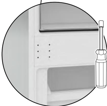
Using a socket screwdriver, remove the hinges and screw them into their new locations to create the thread.
