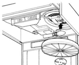
To replace the charcoal filter, support the filter with one hand, remove the round disk through the centre of the charcoal filter and rotate it till the filter will come away .
