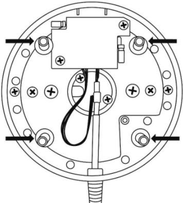
You can also use the 4 holes located in the corners of the metal base plates of the joystick and the throttle to attach both elements to a fixed support.
