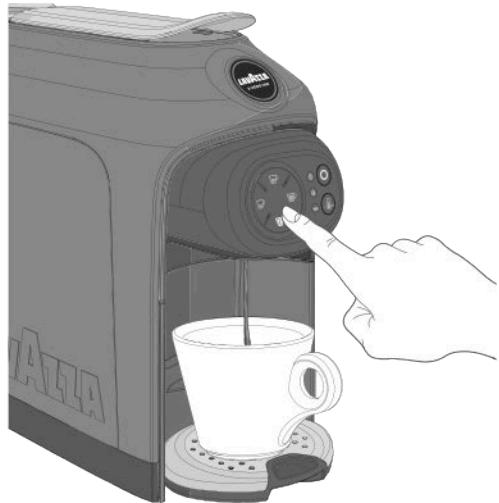
**i** The supply button will light up to a blinking white light when the product is being supplied. You can stop supplying by pressing the supply button again.
