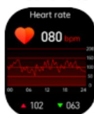
Selecting the Heart Rate interface will start the real-time measurement of your heart rate. The high and low heart rate values measured during the day will also be indicated.
