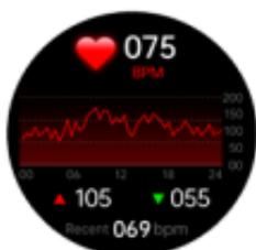
Selecting the Heart Rate interface will start the real-time measurement of your heart rate. The high and low heart rate values measured during the day will also be indicated.
